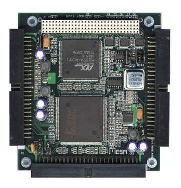
All I/O pins support DCI programmable termination. DCI reference resistance it 100 Ohms.
