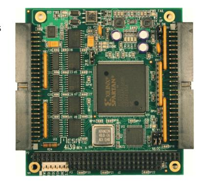
The MESA 4I39 is a communication oriented programmable I/O card for the PC/104 bus. The 4I39 has 8 full duplex RS-422 /485 interfaces that are isolated from PC/104 ground and 24 general purpose TTL I/O pins.
