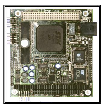
An external IDE interface is also provided. IDE interfaces are PCI based or high performance.
