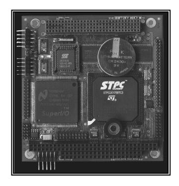
Standard I/O include two 16C550 compatible RS-232 serial ports. One of the ports can be configured for RS-485 type interface.
