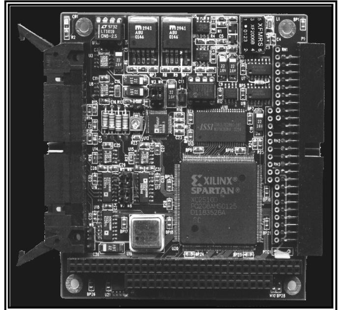
The 4A24 is a high resolution, high speed, low cost A-D card for the PC/104 bus. 200 KHz and 500 KHz models are available. On card EEPROM calibration storage and fully digital zero and span calibration eliminates potentiometers and simplifies circuitry.
