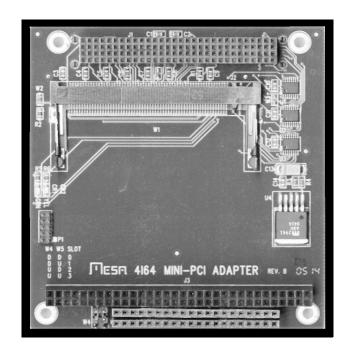
The 4I64 is a type III Mini-PCI adapter for the PC/104-PLUS bus . The 4I64 allows use of Mini-PCI cards like IEEE 802.11 wireless LAN cards and network/modem cards in a PC/104-PLUS system.
